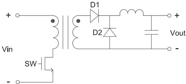
Fig.4: Typical Single Switch Forward Converter Circuit Diagram
