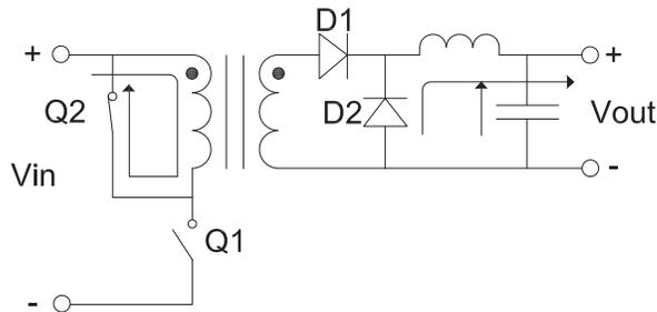
Fig.3: Current Flow w/ Q2 Closed, Q1 Open
