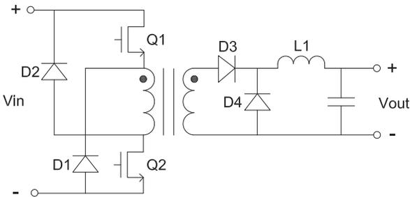
Fig.7: Typical 2-Switch Forward Converter
