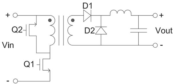
Fig.1: Typical Active Clamp Forward Converter Circuit Diagram
