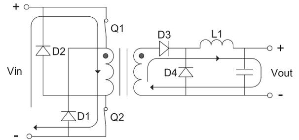
Fig.8: Current Flow w/ BOTH Switches
