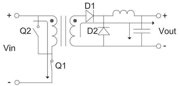
Fig.2: Current Flow w/ Q1 Closed, Q2 Open
