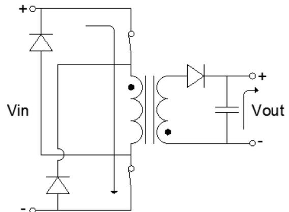
Fig. 5: Current Flow w/ Both Switches Closed-
