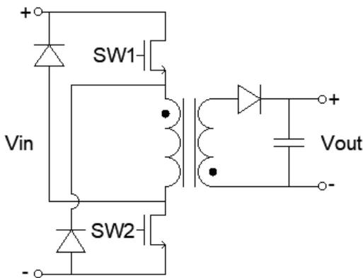
Fig. 4: Typical 2-Switch Flyback Converter
