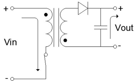
Fig. 2: Current Flow w/ Switch Closed
