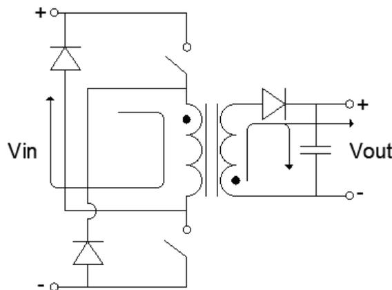
Fig. 6: Current Flow w/ Both Switches Open-
